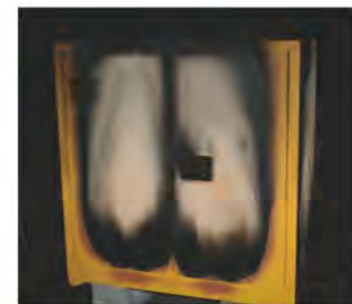
▲ Actual fire exposure testing photo for safety cabinet conducted by FM.
